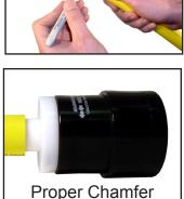
Stab pipe completely into fitting entrance.
